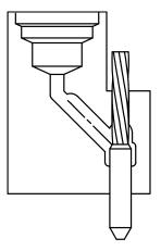
For 4/0 cable and smaller, place end of ground rod to center of tap hole. Butt cable against top of ground rod.
