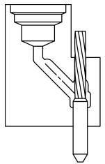
For cables larger than 4/0, place end of ground rod to bottom of tap hole. Butt cable against top of ground rod.
