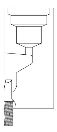
1. Push formed terminal (bond-end) into the mold until it stops
