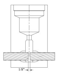
When both cables are larger than 750 MCM, gap cables 1/8" under center of tap hole.
