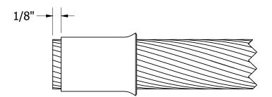
3) Position the cable with sleeve into the mold such that the sleeve cannot slide in any further into the mold.
