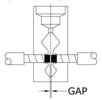
3. Place the conductors into the mold with a gap between the ends centered on the tap hole.
