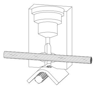
Place cable into mold. For cables larger than 300 MCM, cut and gap 1/4" under center of tap hole. Follow instructions on reverse side for proper use of packing material.
