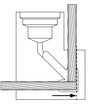
Align end of horizontal cable with side of vertical cable and butt vertical cable against horizontal cable. Do not allow end of horizontal cable to protrude past side of vertical cable.
