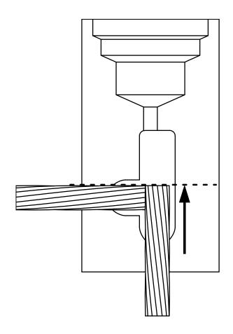
Align end of vertical cable with upper edge of horizontal cable and butt horizontal cable against vertical cable.
