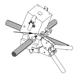
Place tap cable over run cable. Cables are uncut. To remove mold more easily from finished weld: unscrew top thumbscrew of mold handle. Re-fasten mold handle thumbscrew prior to next connection.
