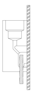
Place end of cable to bottom of tap hole. Secure mold to surface using CSKITVPH3 chain support, MSKITH3 magnetic support, or a C-Clamp.
