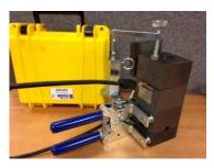
**Step 6 :** Make sure filter housing is seated firmly on mold then apply pressure to filter housing using hold down screw. Position hold down screw over igniter.
