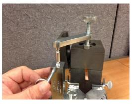
**Step 7 :** Attach US controller and ignite shot and make an UltraShot Connection per Instructions
