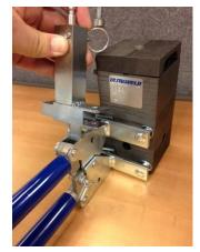
Step 2 : Line up holes and replace Tab Pin
