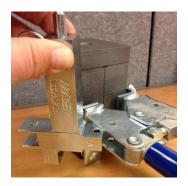
**Step 3 :** Follow mold instructions for placement of conductors in Mold and place appropriate size UltraShot Cartridge in the mold with igniter tab in slot in mold.
