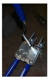
Step 3: Insert MH1 handle clamp with UMHDKIT into mold and tighten thumb screw.
