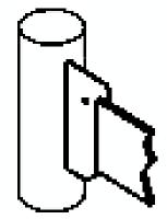
**Important:** A test weld should be made to check the possibility of burn through on thin metal or thin wall pipe. On thin wall fence posts, filling the post with sand well above the location of the weld may reduce burn through problems. Other solutions would be to use a smaller conductor or utilize mechanical connections.
