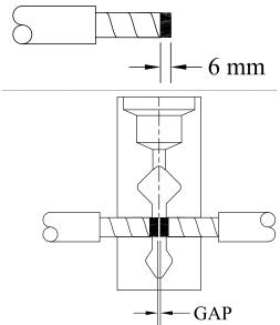
3. Place the conductors into the mold with a gap between the ends centered on the tap hole.
