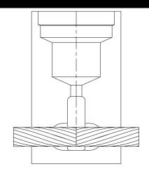
Butt cables under center of tap hole for 400 mm<sup>2</sup> and smaller.
