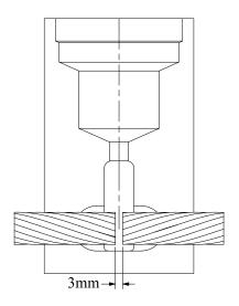
For 500 mm<sup>2</sup> and larger, gap cables 3 mm under center of tap hole.
