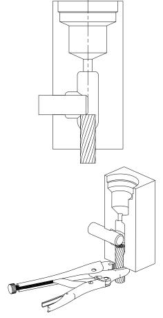
Place end of ground rod under the center of the tap hole. Ground rod must sit on top of cable. Use locking pliers or a clamp on the cable below the mold to prevent it from slipping when the mold is fired.
