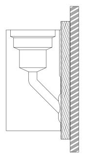
Place cable in mold and secure on surface using CSHI chain clamp, MSHC magnetic clamp, or C clamp. Packing material is required for 1/0 and larger cable to prevent leakage between cable and steel surface.
