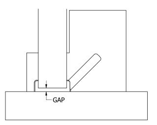
Align upper edge of horizontal bus bar with slot in mold and place vertical bus bar in mold. Bus bars 1/8" thick and thinner are gapped 1/8". Bus bars thicker than 1/8" are gapped 1/4".
