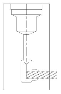
Place end of cable under the center line of the tap hole. Secure to surface ushing CSH1 chain clamp, MSHC magnetic clamp ora a C clamp. Pack openeing with packing material when necessary.
