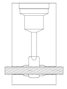
Place cable in mold and secure on surface using CSHI chain clamp, MSHC magnetic clamp, or C clamp. Packing material is required for 1/0 and larger cable to prevent leakage between cable and steel surface.
