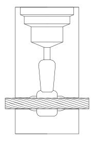
Place cable in mold and secure on surface using CSHI chain clamp, MSHC magnetic clamp, or C clamp.
