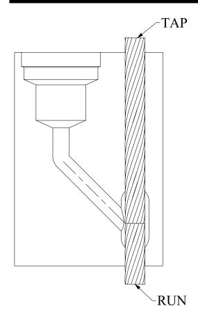
Place end of lower cable to center of tap hole, then butt upper cable against lower cable
