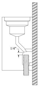
Place end of cable as far up into the mold as possible, then pull cable out ¼". Secure mold to surface using CSHI chain clamp, MSHC magnetic clamp or a C clamp.
