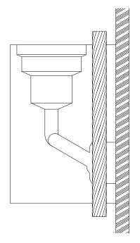
Place cable in mold and secure on surface using CSHI chain clamp, MSHC magnetic clamp, or C clamp.
