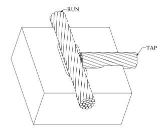
Place run cable into mold. Butt tap cable against run cable.
