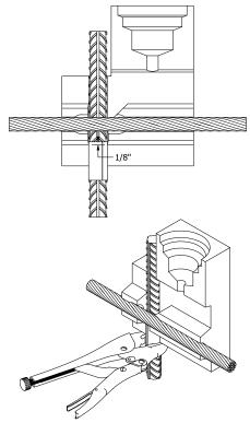
Place cable and reinforcing bar into the mold. Do not run cable through mold.
