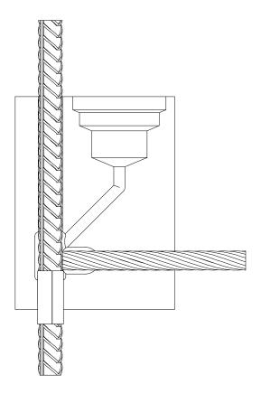
Position cable against reinforcing bar in mold.
