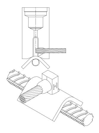
Place end of cable to the center of tap hole
