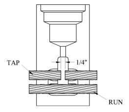
If TAP cable is larger than 300 MCM, cut & gap ¼" under center of tap hole. Do not cut for heavy duty molds.
