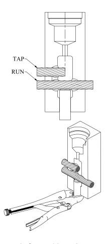
Place end of tap cable under center of tap hole. Run cable must sit on top of the ground Rod. Use locking pliers or a clamp on the rod below the mold to prevent it from slipping when the mold is fired.
