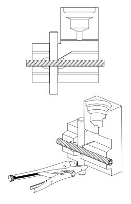
Place cable into mold and secure mold to ground rod with handle clamp. Use locking pliers or a clamp on the rod below the mold to prevent it from slipping when the mold is fired.
