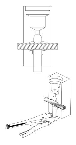
Place cable in the mold. Cable must sit on top of ground rod. Use locking pliers or a clamp on the rod below the mold to prevent it from slipping when the mold is fired.
