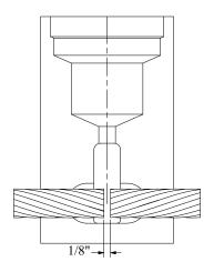
For 800 MCM and larger, gap cables 1/8" under center of tap hole.
