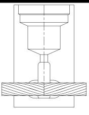
Butt cables under center of tap hole for 750 MCM and smaller.
