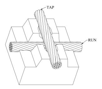
Place tap cable over run cable. Cables are uncut.
