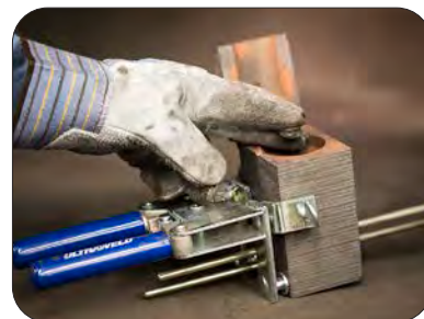
Step 3: Insert disk into mold.
