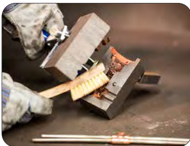
Step 7: After the connection is complete, open the mold and remove the connection, remove slag and clean mold before making the next connection.
