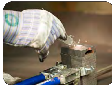
Step 6: Ignite material located on top of the lid using a flint igniter (FLTIG).
