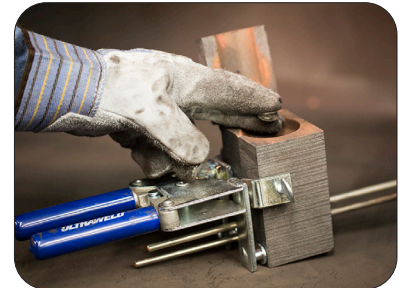
Step 3: Insert disk into mold.
