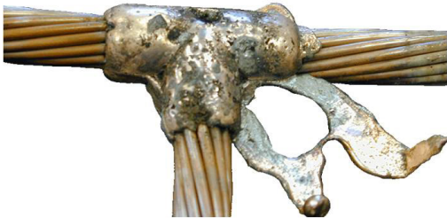
Weld was not closed properly or it was worn out and leaked significantly. Also there is too much slag in the weld. Replace mold if needed.
