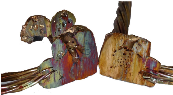
The above weld cut in half reveals the amount of voids in the weld. These can be caused by contaminates in the mold, conductor or weld metal. Note: A small number pin holes are acceptable, up to 20%.
