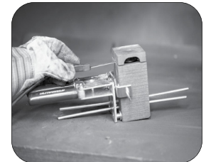
Step 3: Close the lid and attach DRONE cord to the UltraShot igniter.
