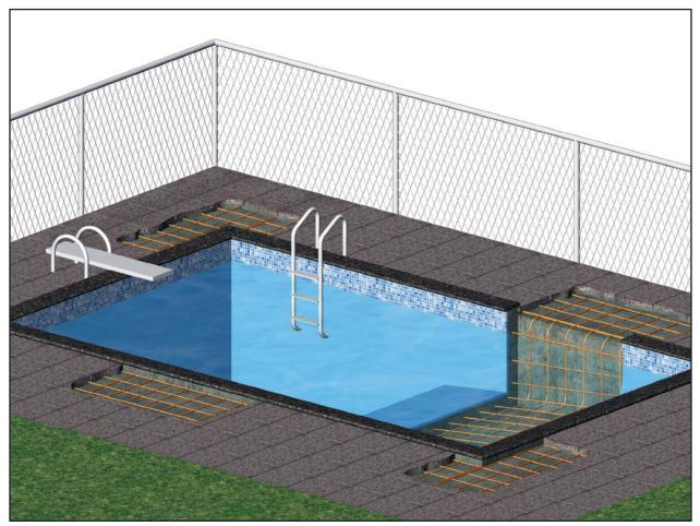
**Voltage Gradient Control** Ground Mesh is used to reduce Voltage Gradients in the pool area.
