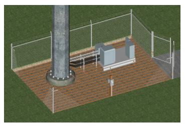
**Equipotential Plane** Provides equipotential ground plane in environments with little top soil where standard ground systems are not feasible.
