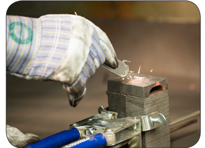
Step 6: Ignite material located on top of the lid using a flint igniter (FLTIG).
