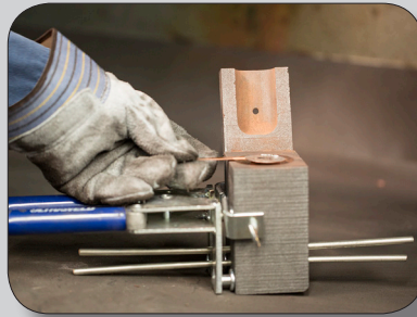
step 2 Place conductors and UltraShot cartridge into mold.
