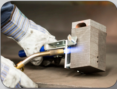
step 1 Dry and Clean the mold and conductor.
